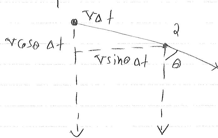
Suppose we observe a blob of relativistic electrons emitting synchrotron radiation as they move from point 1 to point 2 in the above figure. The apparent duration of the pulse received
